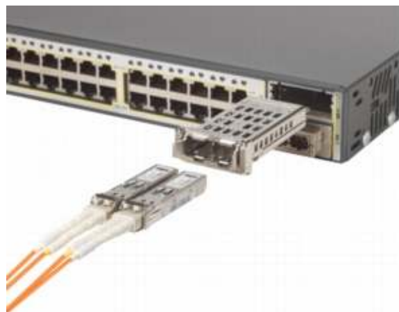
Figure 2. Cisco TwinGig Converter Module Converts a 10 Gigabit Ethernet X2 Interface into Two Gigabit Ethernet SFP Ports in the Catalyst 3750-E and Catalyst 3560-E Series Switches.
