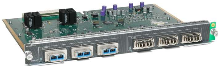
Figure 5. Cisco TwinGig Converter Module converts each 10 Gigabit Ethernet X2 Interface into Two Gigabit Ethernet SFP Ports with Catalyst 4500 E-Series 6-port 10 Gigabit Ethernet Linecard
