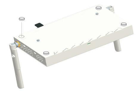
Mounting on a wall – The access point should be mounted only to a wall or wood surface that is at least 1/2-inch plywood or its equivalent. To mount the access point on a wall, always use its wall-mounting bracket.
