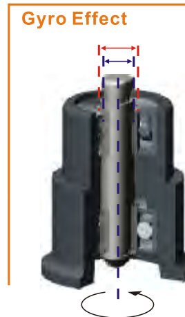
The Gyro Effect Short the Life of Bearing and More Vibration Unstable!
